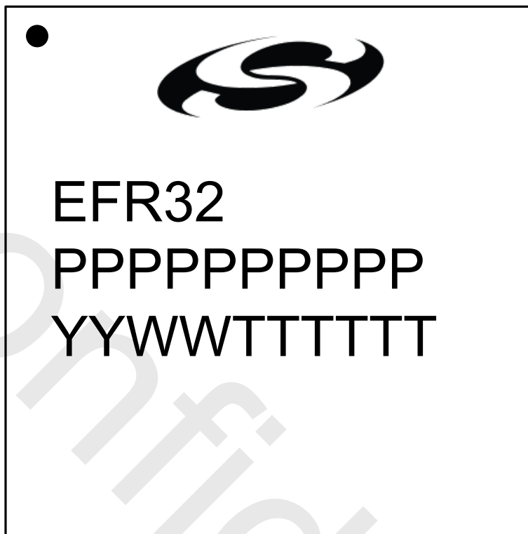
Figure 8.3. QFN48 Package Marking
