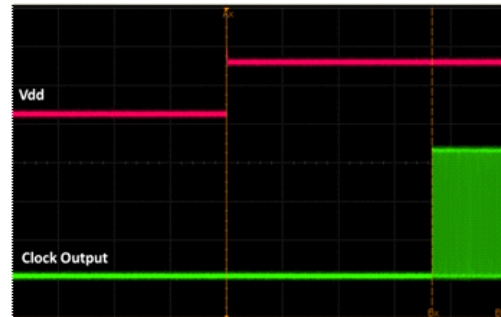
Figure 17. Startup Waveform vs. Vdd
