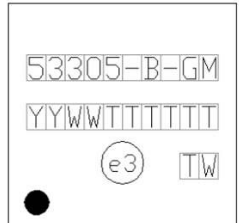
Figure 8.6. Si53305 Top Marking
