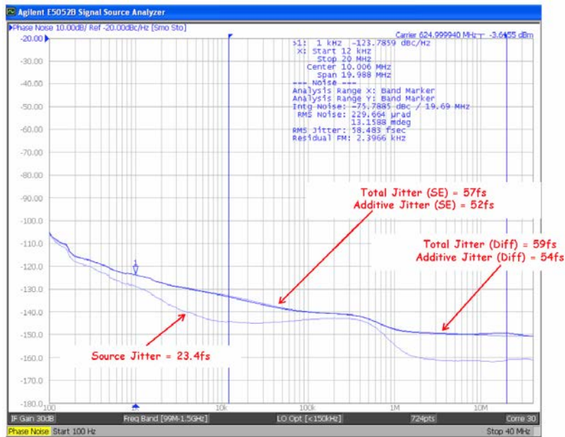
Figure 2.15. Total Jitter Differential Input (312.5 MHz)
