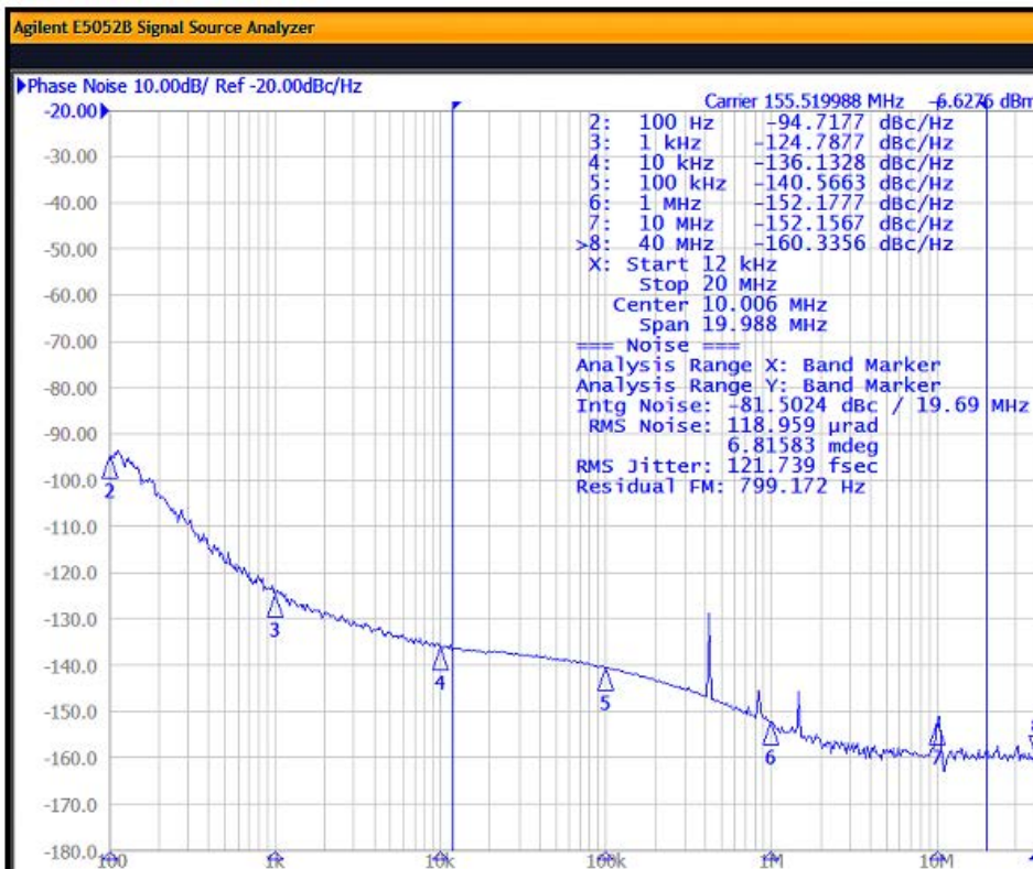
Figure 8.3. Input = 25 MHz; Output = 155.52 MHz, 2.5 V LVDS
