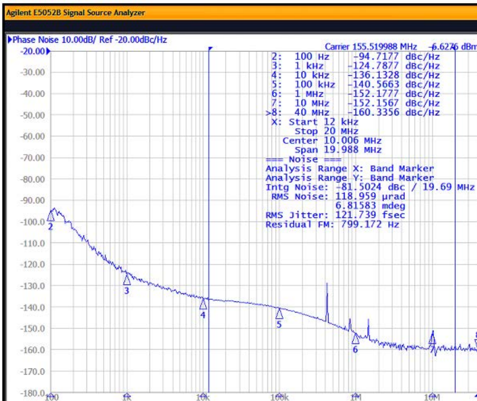
Figure 8.3. Input = 25 MHz; Output = 155.52 MHz, 2.5 V LVDS
