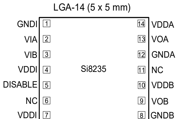
Figure 44. Si8235 LGA-14 (5x5 mm) Pinout
