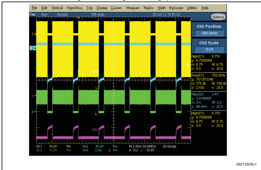
Figure 25: Inverting BB dimming operation
