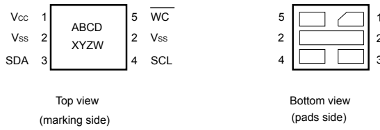
Figure 3. UDFPN5 (DFN5) package connections
