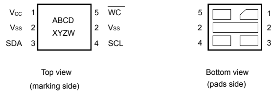
Figure 3. UFDFPN5 (DFN5) package connections
