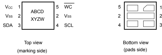
Figure 3. UFDFPN5 (DFN5) package connections
