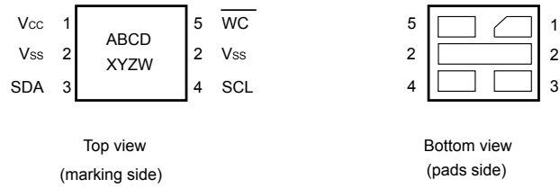
Figure 3. UFDFPN5 (DFN5) package connections
