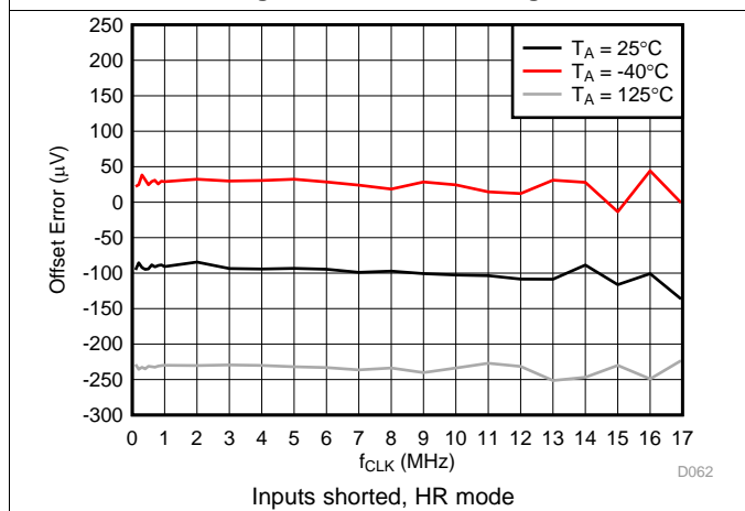
Figure 40. Offset Voltage vs f_{CLK}
