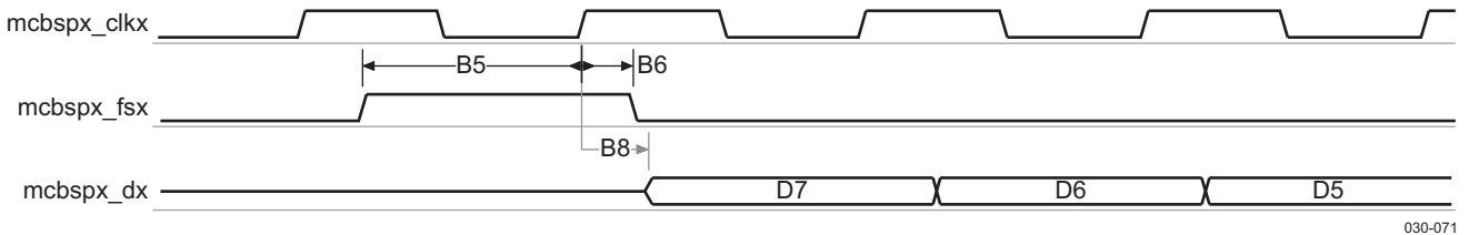
Figure 6-40. McBSP Rising Edge Transmit Timing in Slave Mode
