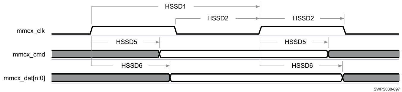
Figure 6-74. MMC2 and MMC3 Interfaces—High-Speed SDIO Mode—Data/Command Transmit (1)
