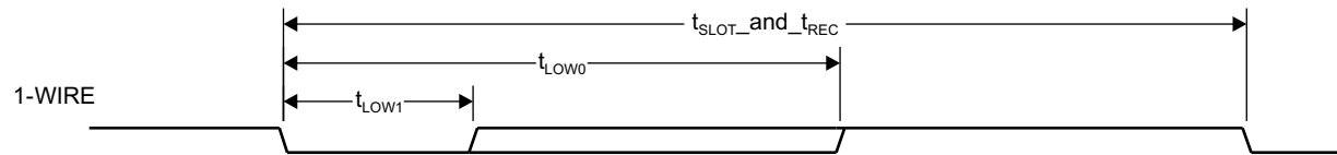
Figure 5-118. 1-Wire Write Bit Timing (Command/Address or Data)
