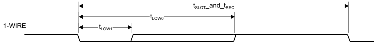
Figure 5-118. 1-Wire Write Bit Timing (Command/Address or Data)
