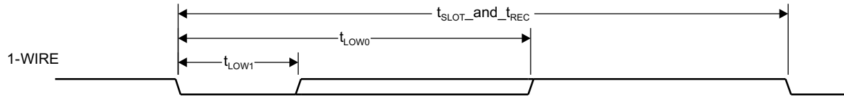
Figure 5-118. 1-Wire Write Bit Timing (Command/Address or Data)
