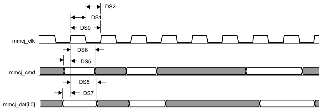
Figure 7-81. MMC/SD/SDIOj in - Default Speed - Receiver Mode
