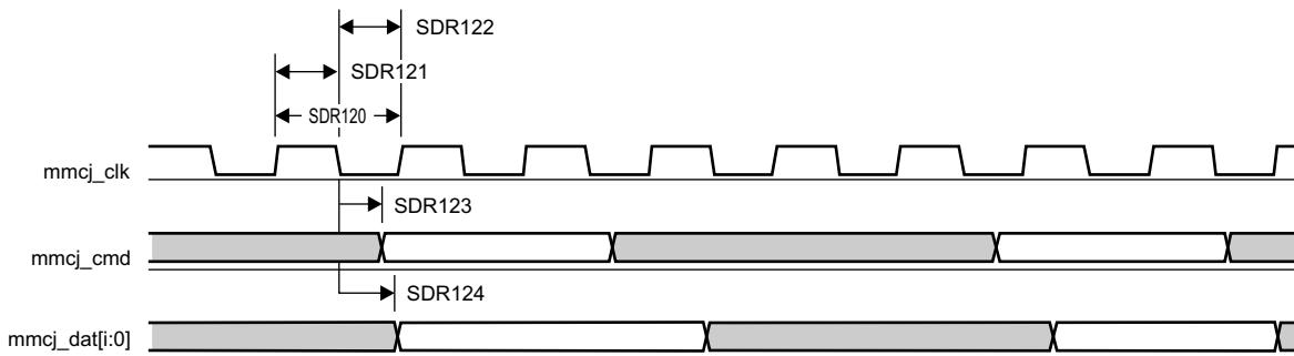
Figure 7-86. MMC/SD/SDIOj in - SDR12 - Transmitter Mode
