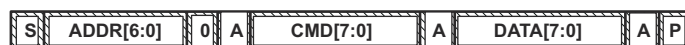
Figure 7-3. Attempt To Write a Read-Only Address (Nack After Data Sent By Master)
