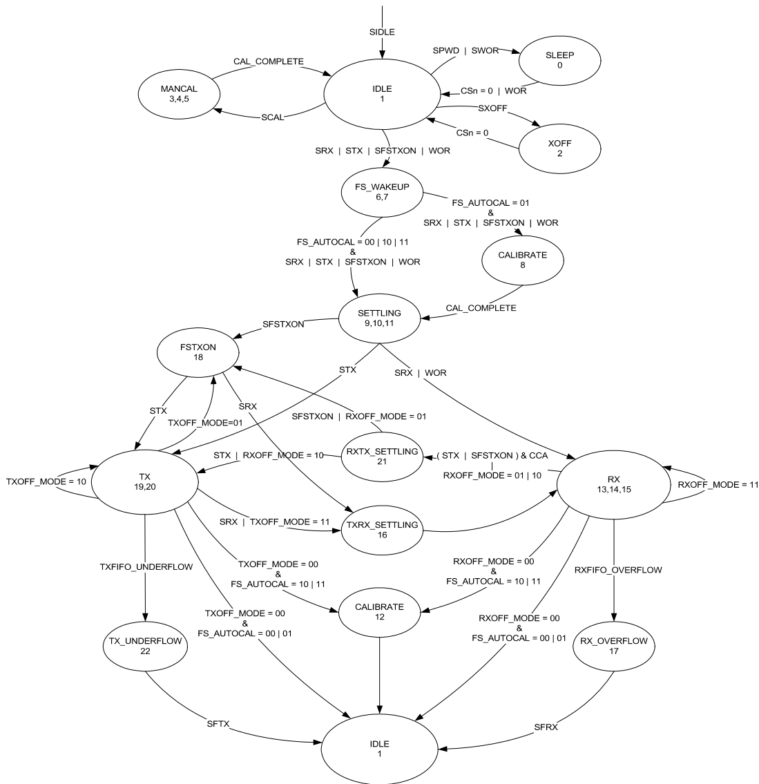
Figure 25: Complete Radio Control State Diagram
