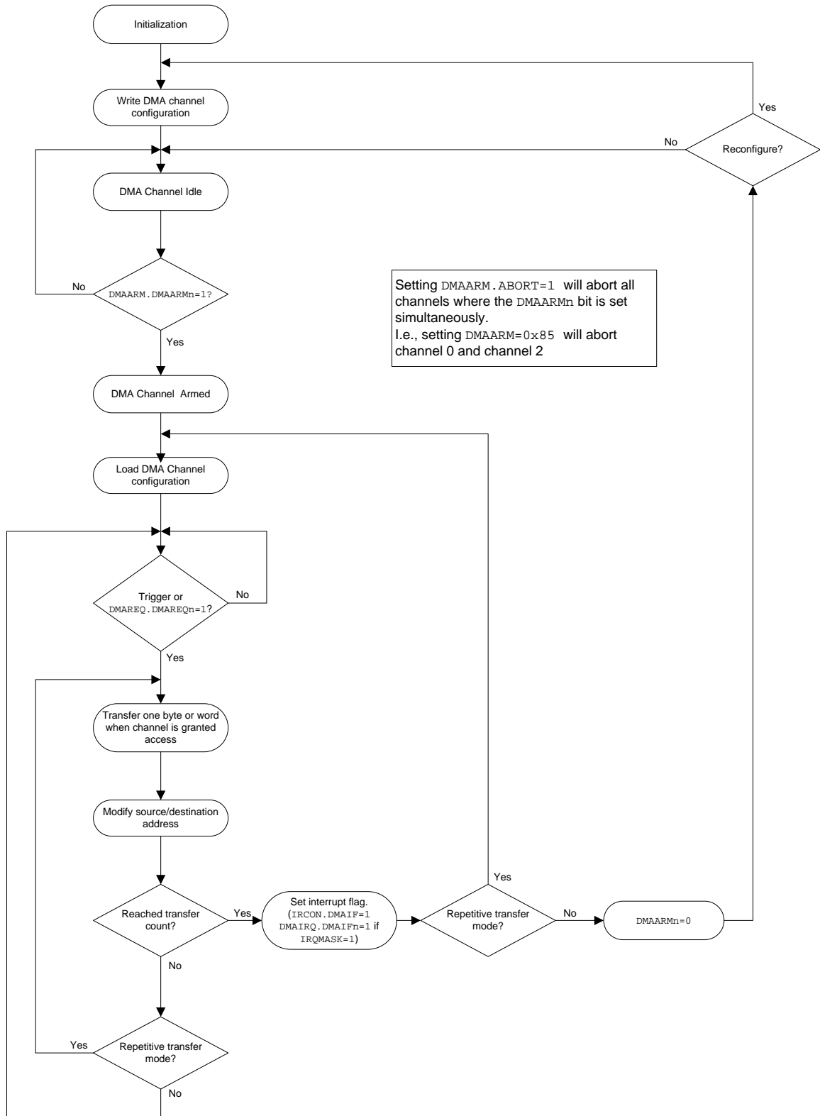
Figure 26: DMA Operation
