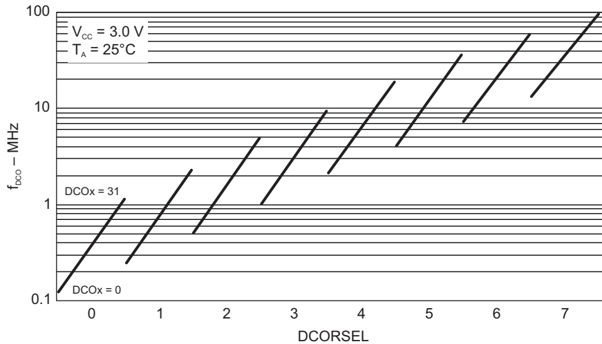
Figure 5-13. Typical DCO Frequency
