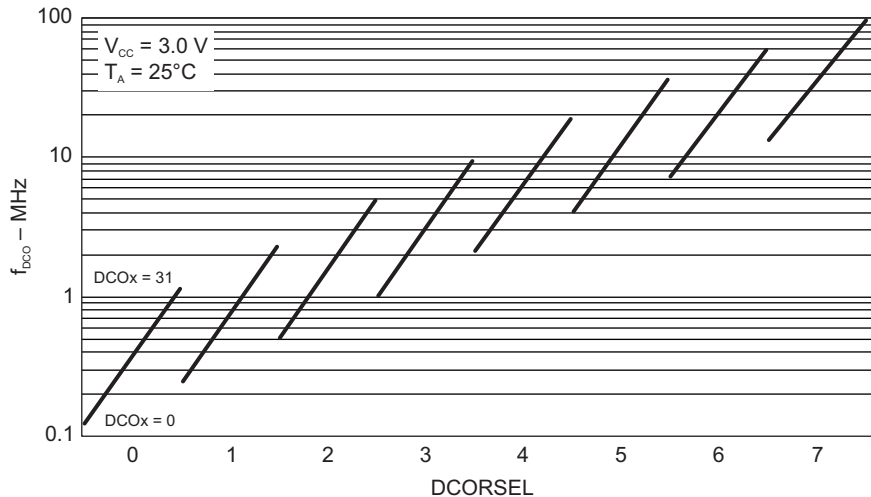
Figure 5-13. Typical DCO Frequency
