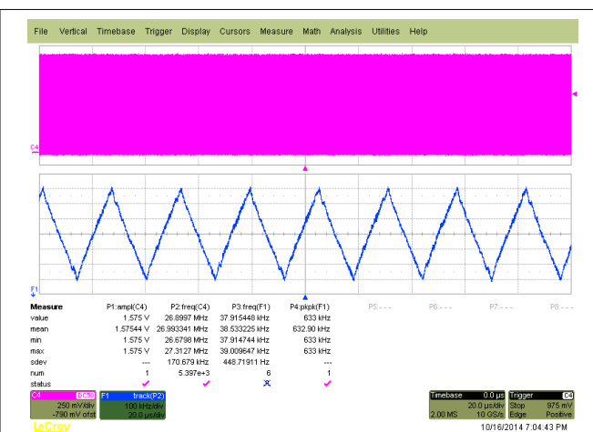
Figure 9-7. f_{OUT} = 27\text{MHz} , VCO Frequency > 175MHz, SSC (1%, Center)
