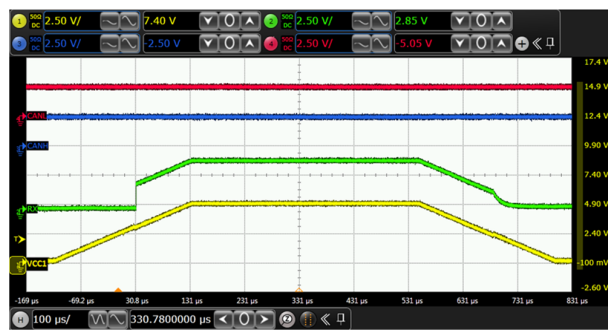
Figure 6-11. V_{OD(DOM)} Over V_{CC}
