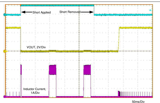
Figure 8-6. Short-Circuit Transient and Recovery
