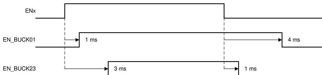
Figure 10. Typical Start-Up and Shutdown Sequencing
