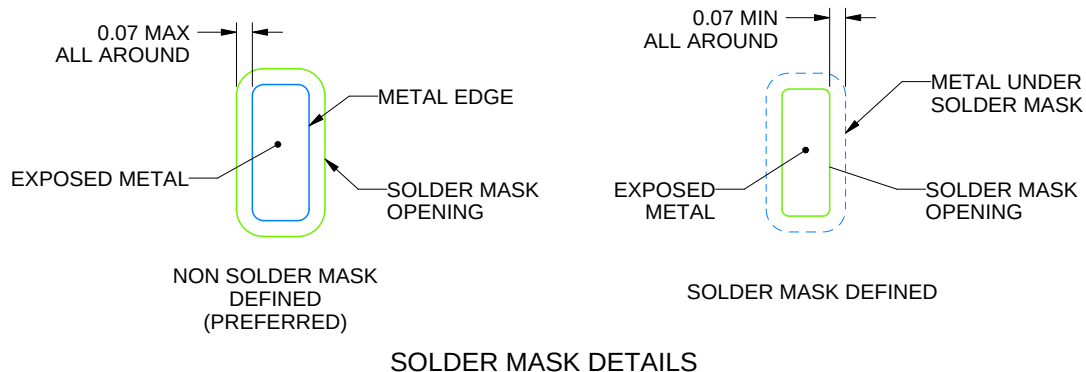
LAND PATTERN EXAMPLE EXPOSED METAL SHOWN SCALE: 10X
