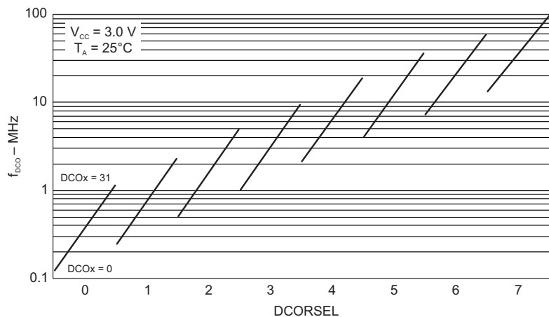
Figure 5-10. Typical DCO Frequency
