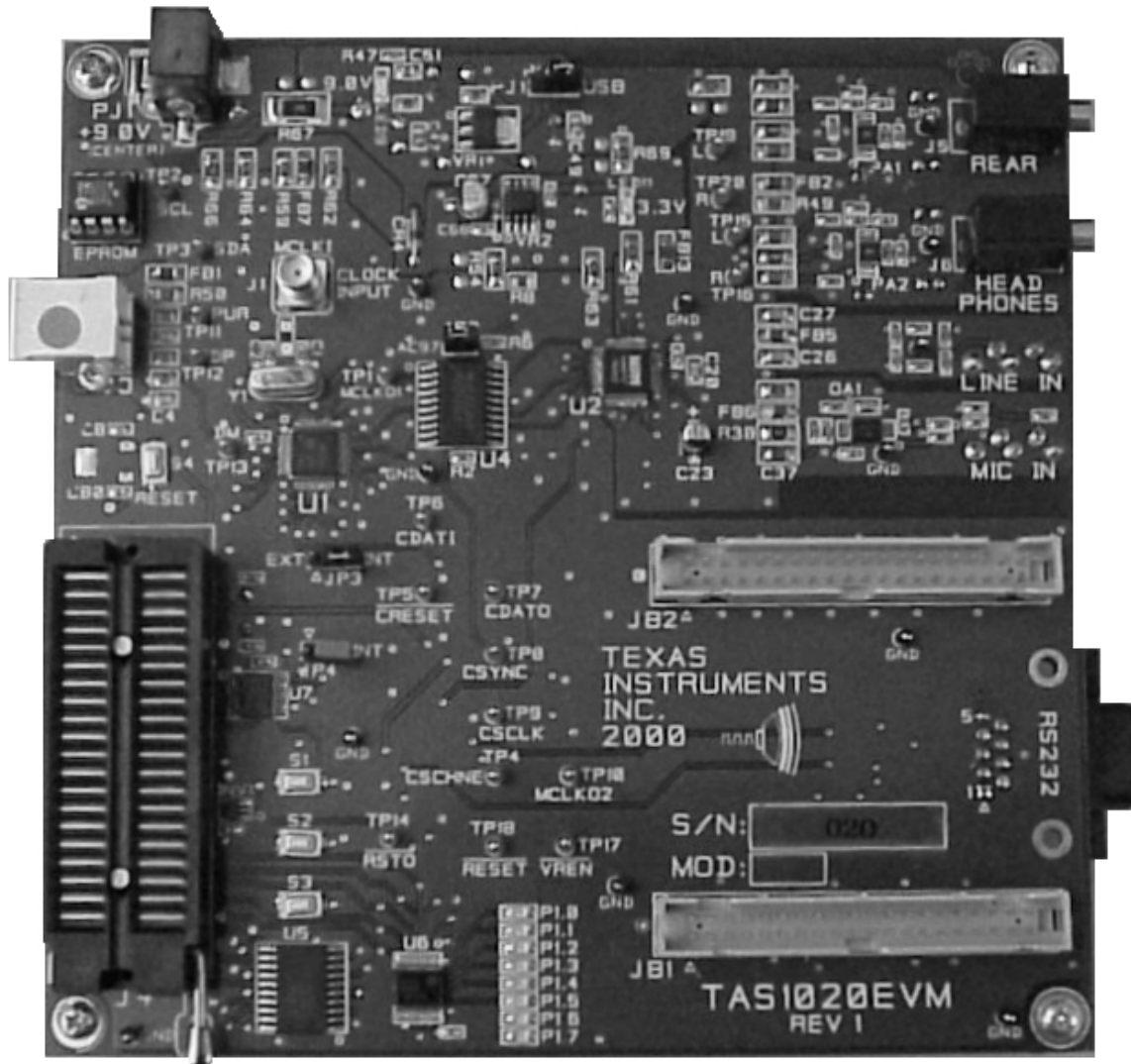
Figure 2–1. TAS1020A EVM Top View
