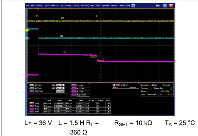
Figure 9-6. CQ Driving Inductive Load, Low Side Mode (NPN mode)
