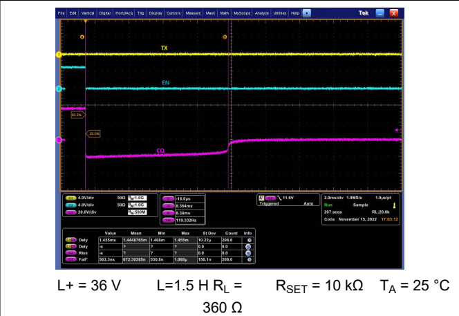
Figure 9-7. CQ Driving Inductive Load, High Side Mode (PNP mode)
