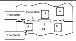
(3) Mounting components near screw holes
