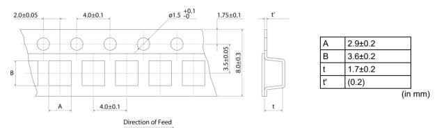
\* The dimensions of the cavity are measured at its bottom.
