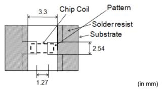
Do not use gilded pattern. A copper wire may cause open by dissolution of metallization.
