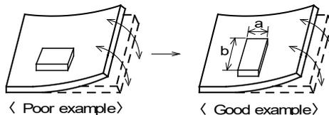
(2) Components location on PCB separation
