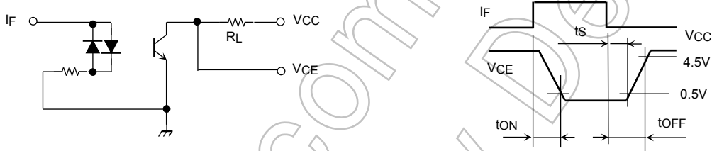
Fig. 1: Switching operating conditions
