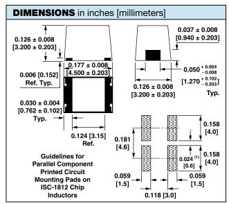
(1) Recommended minimum spacing between components
