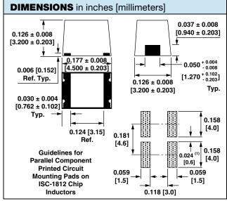
(1) Recommended minimum spacing between components
