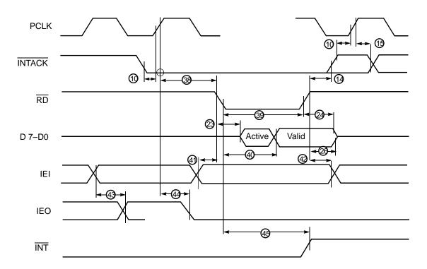
Figure 31. Z85230/L Interrupt Acknowledge Timing Diagram
