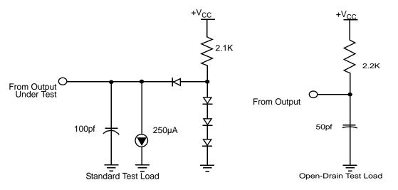
Figure 23. Standard and Open-Drain Test Loads
