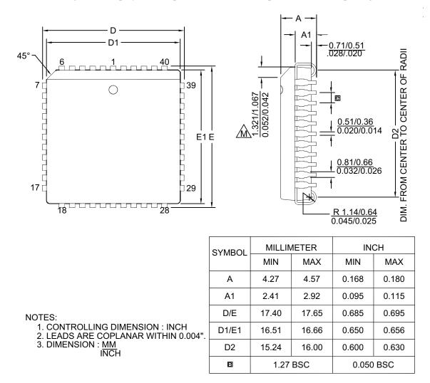
Figure 38 displays the 44-pin Plastic Leaded Chip Carrier (PLCC) package.
