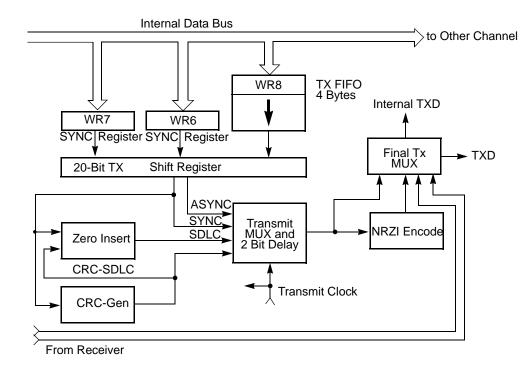
Figure 5. ESCC Transmit Data Path
