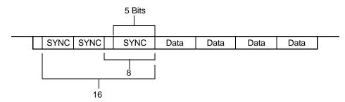
Figure 9. Detecting 5- or 7-Bit Synchronous Characters
