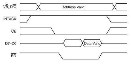
Figure 20. Read Cycle Timing (Z85230/L)
