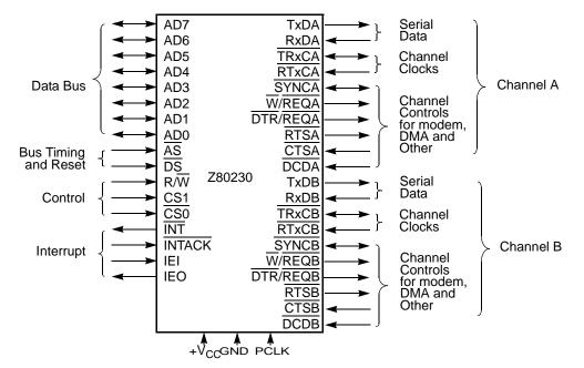
Figure 2. Z80230 Pin Functions
