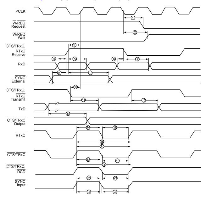
Figure 27 displays the Z80230 general timing diagram.
