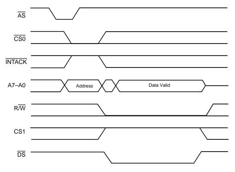
Figure 17. Z80230 Write Cycle Timing
