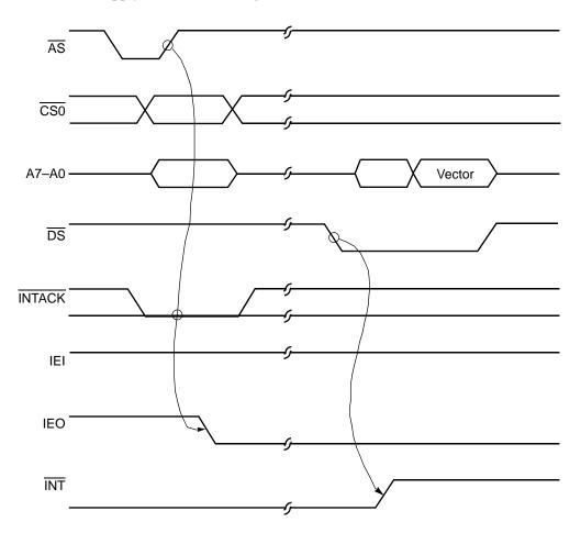
Figure 19. Z80230 Interrupt Acknowledge Cycle Timing
