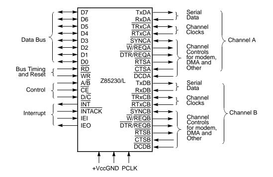
Figure 1. Z85230/L Pin Functions
