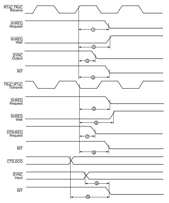
Figure 28 displays the Z80230 system timing diagram.
