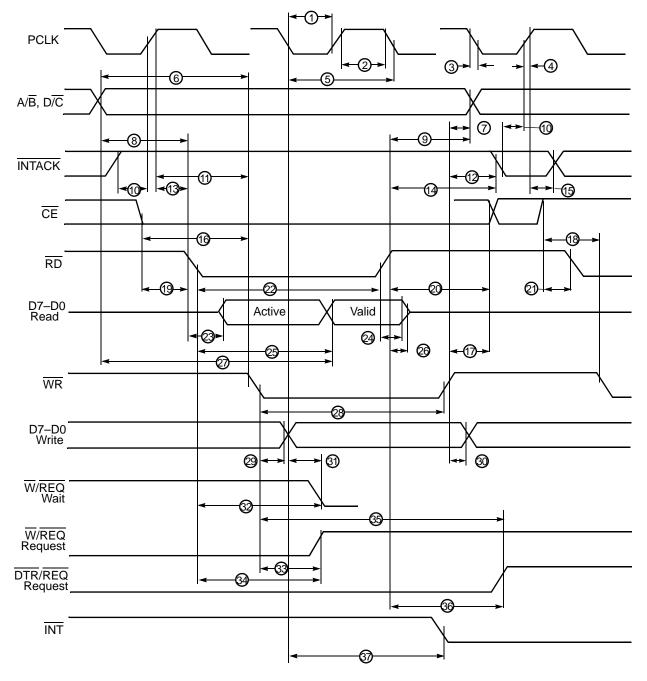
Figure 29. Z85230/L Read/Write Timing Diagram
