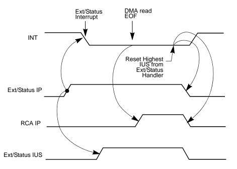
Figure 35 displays the procedure for resetting highest IUS.
