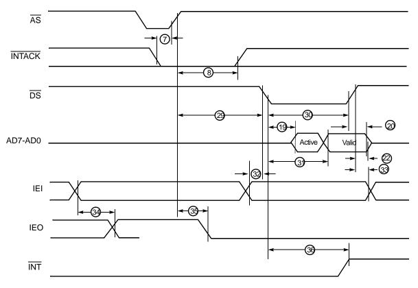
Figure 25 displays the Z80230 Interrupt Acknowledge timing diagram
