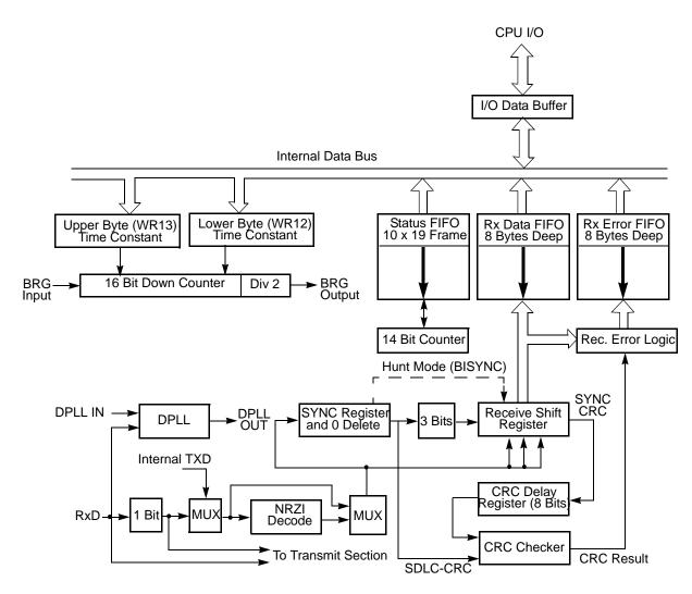
Figure 6. ESCC Receive Data Path
