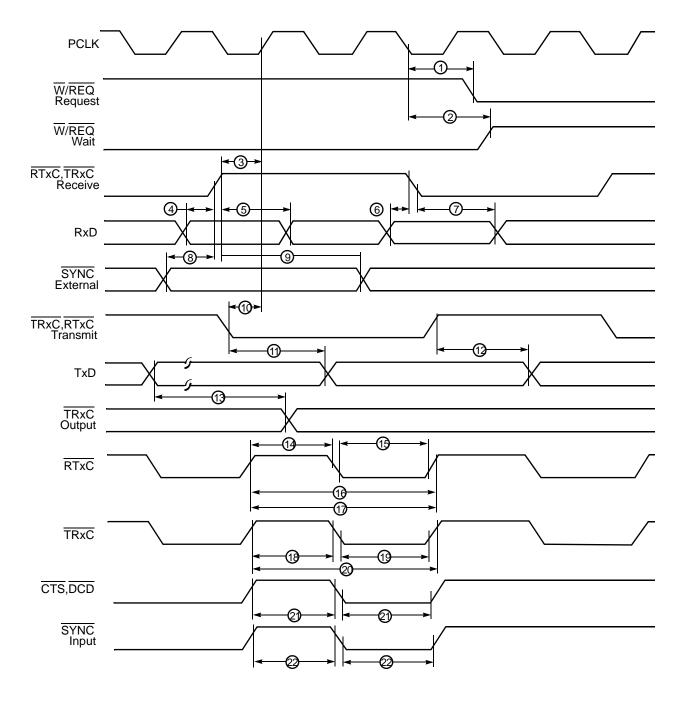
Figure 33. Z85230/L General Timing Diagram
