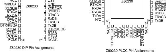
Figure 4. Z80230 Pin Assignments
