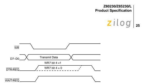
Figure 12. DMA Request on Transmit Deactivation Timing
