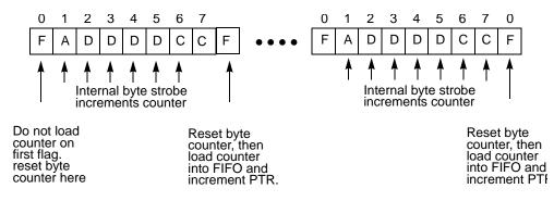
Figure 16. SDLC Byte Counting Detail
