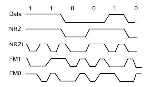
Figure 11. Data Encoding Methods
