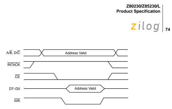
Figure 21. Write Cycle Timing (Z85230/L)
