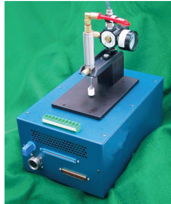
Figure 3-9: \theta_{JC} Measurement Setup
