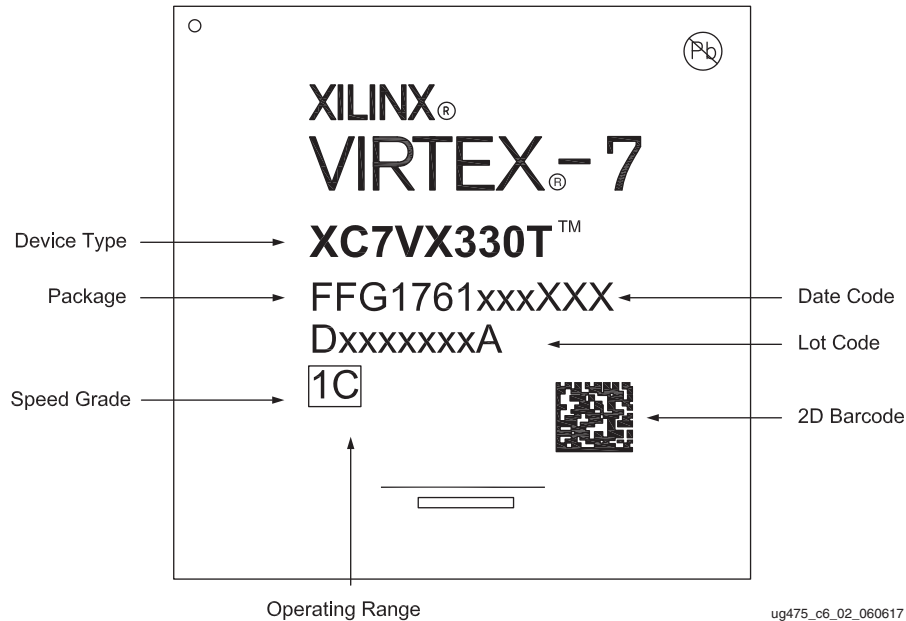
Figure 6-10: Legacy Virtex 7 Device Package Marking
