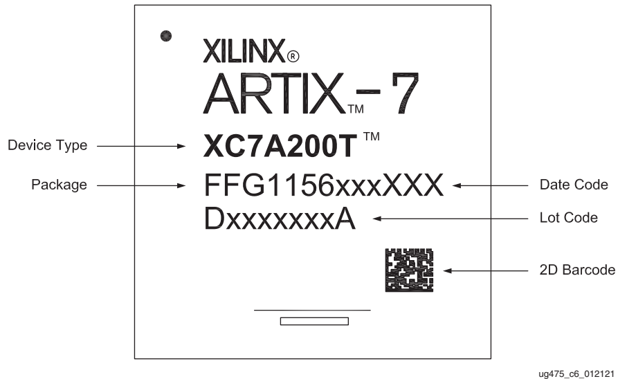
Figure 6-2: Artix 7 Device Package Marking with 2D Bar Code
