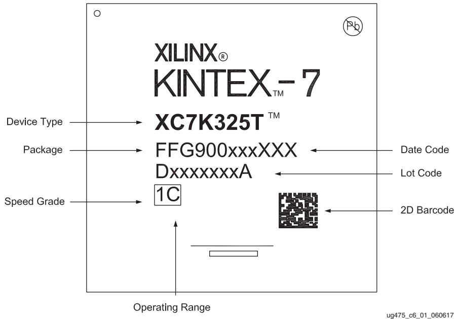
Figure 6-7: Legacy Kintex 7 Device Package Marking
