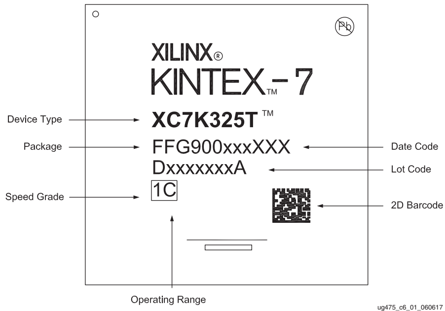
Figure 6-7: Legacy Kintex 7 Device Package Marking
