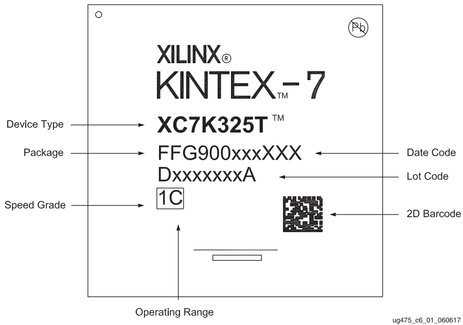
Figure 6-7: Legacy Kintex 7 Device Package Marking
