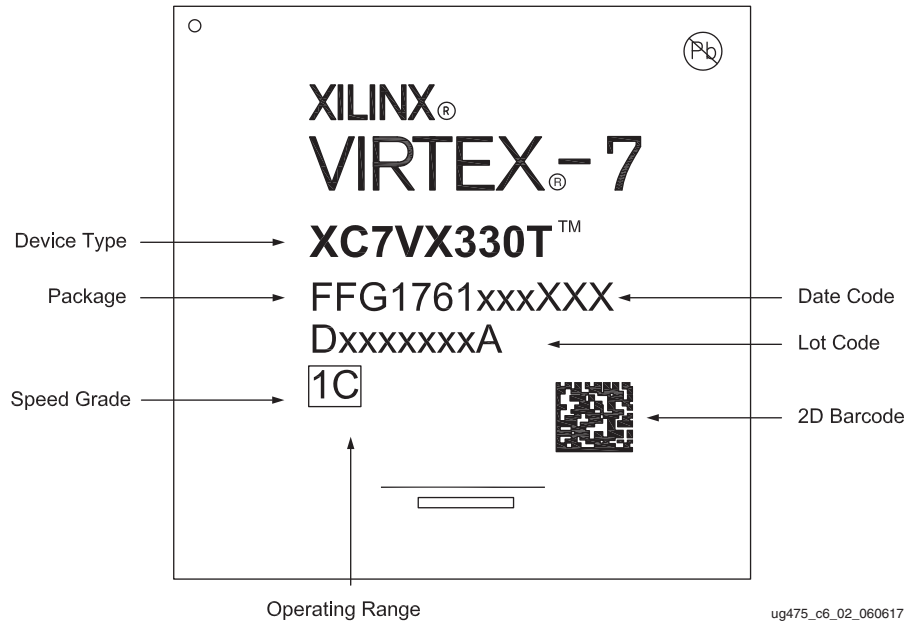
Figure 6-10: Legacy Virtex 7 Device Package Marking
