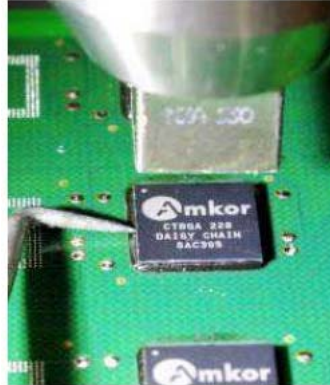
Figure 9-7: Removing Underfill Using Steel Probe
