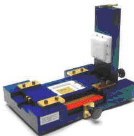
Figure 4-1: Altair BGA Fixture Used for TDR Measurement
