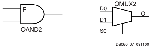
Figure 7: AND and MUX Symbols in Spartan-XL IOB
