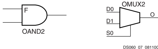
Figure 7: AND and MUX Symbols in Spartan-XL IOB
