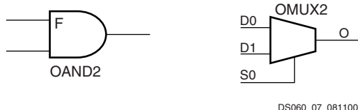
Figure 7: AND and MUX Symbols in Spartan-XL IOB
