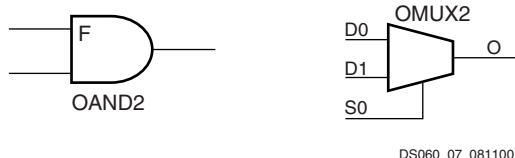
Figure 7: AND and MUX Symbols in Spartan-XL IOB
